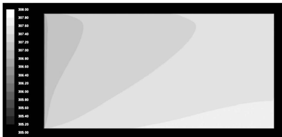
Fig. 3 Temperature distribution in the flat surface of the heat sink fin. Fluid flow is from left to right. Heat flow is from the bottom.
