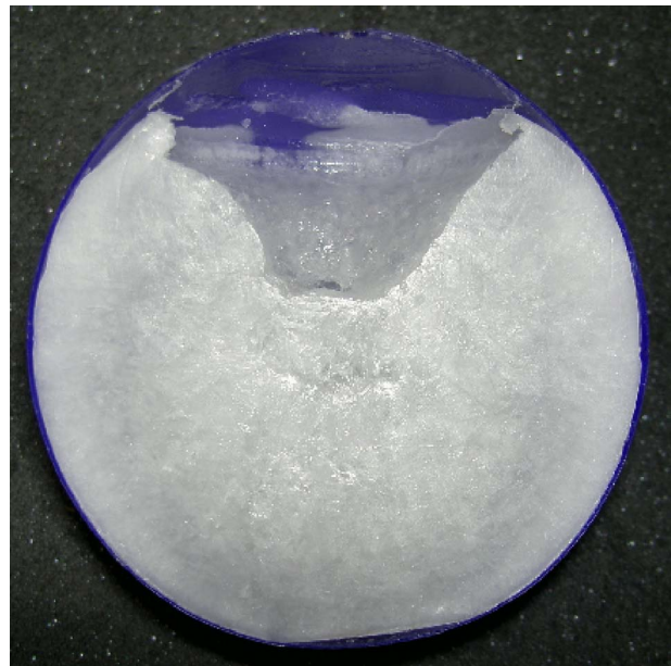
Fig. 2 Solidification with an upper void (shrinkage) for D=70 mm and \Delta T=20 °C [25]
